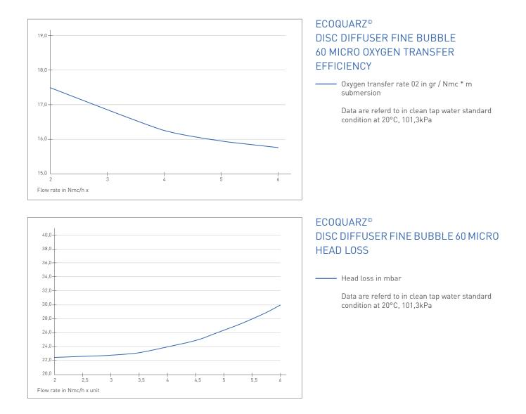
Comparable values can only be optained with a similar setup and condition. Depending on the tank geometry, slit chart, water depth and planar allocation, the quoted values can change. All the data are based on clean water 20° temperature, 1013mbar / 68°F, 101,3kpa. All data are approximate data!
